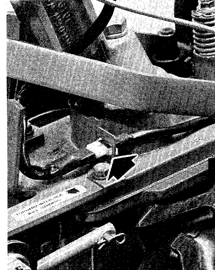
5-13: Forward Interlock Wire Harness.
